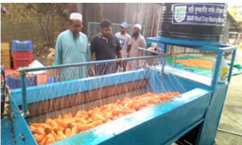
Photo: Washing carrot by BARI root crop washing machine in March 2020
